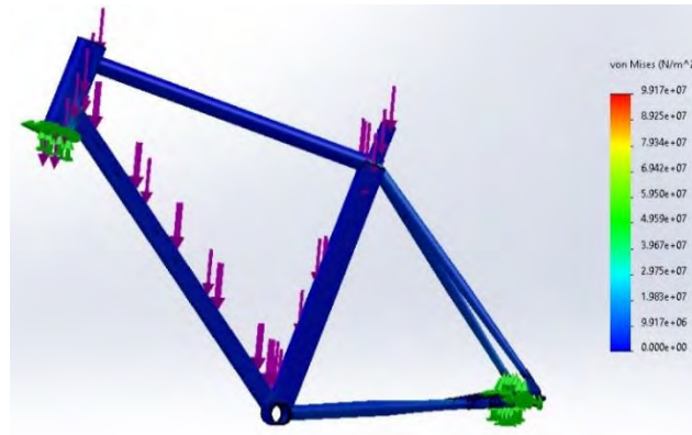
Figure 28: A von Mises stress plot of the interim analysis of the frame (max value 99 MPa).
