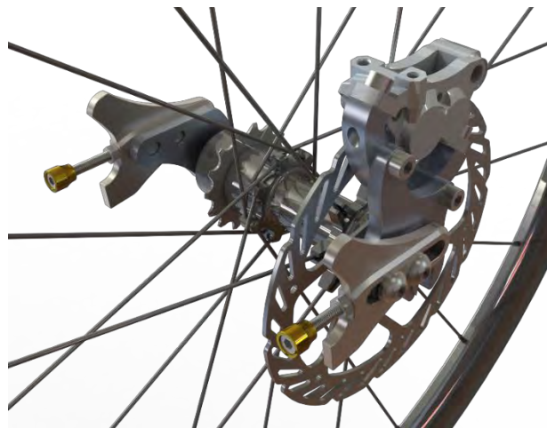
Figure 16: Estimated CAD recreation of commercially available sliding dropouts by Paragon Machine Works, assembled on the rear wheel with disc brake callipers attached.
