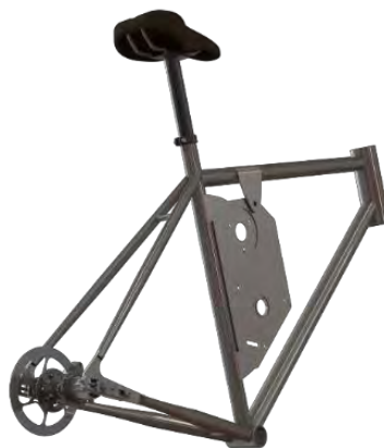
Figure 20. Phase 2 redesigned assembly with proposed motor plate mounting tabs.
