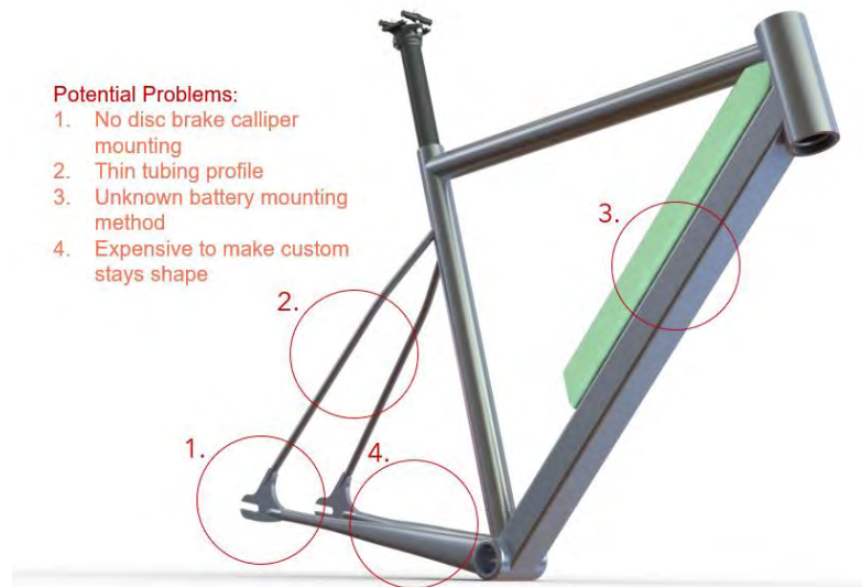
Figure 15. Second iteration of frame design annotated with remaining problems.
