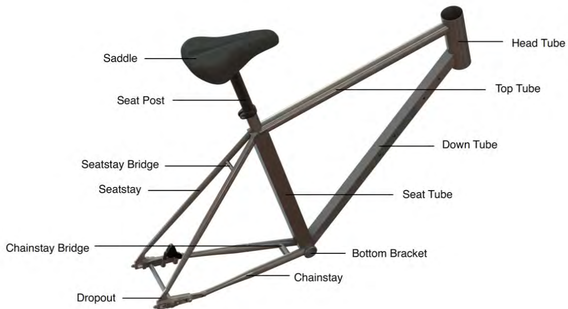
Figure 1: General Terminology for Frame Components.
