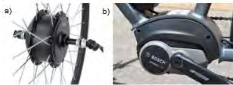
Figure 2: a) A commercially available hub motor mounted on the rear wheel (Direct Voltage n.d.) and b) A mid drive motor solution by Bosch demonstrating the additional complexity of the frame design (Mikey G, 2019).
